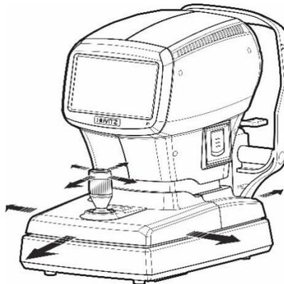
**[Operating the joystick for left/right & focus adjustment]**
